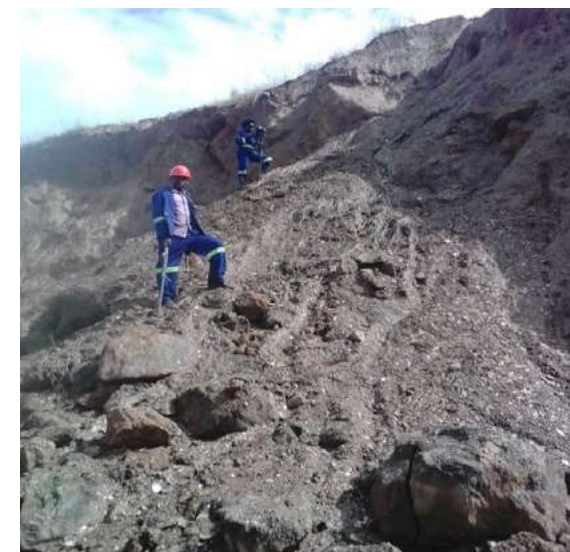
Figure 5: Surveyor picking topographic data for volume reconciliation, Namekara mining company, Manafwa
